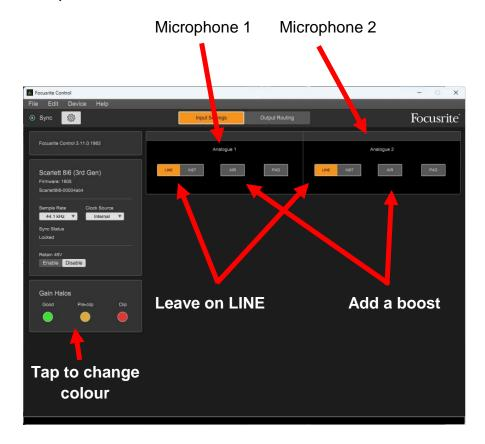
If microphones are plugged into the front channels 1&2, they will be represented as *Analogue 1&2* in the app. If instruments are plugged into
